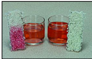
Without stain resistance – raw carpet is permanently stained
